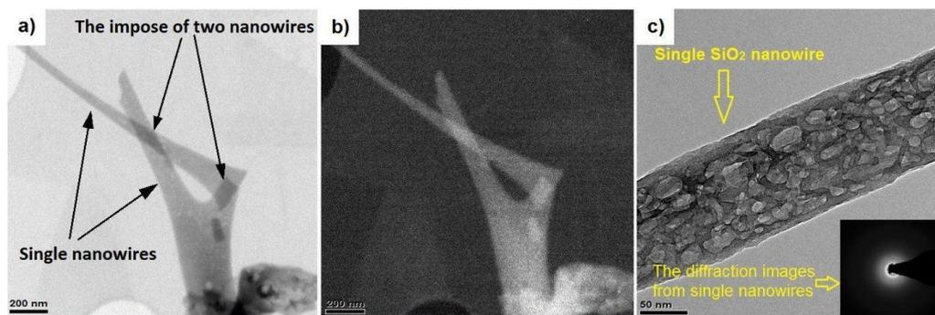
**Figure 3** TEM images of the tested nanowires SiO<sub>2</sub> (obtained from the second spinning solution): a) an image in a light area, b) an image in a dark area, c) a diffraction image from single nanowires obtained using analytical electron microscopy in nanoareas in STEM.
