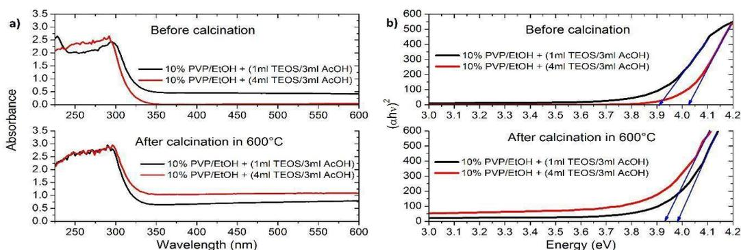
**Figure 4** UV-Vis spectrum (a) and dependencies  $(\alpha h\nu)^2$  as a function of energy quanta of radiation, along with matching straights, crossing of which with energy axis corresponds to breaks values (b) obtained for the composite nanofibers PVP/SiO<sub>2</sub> (before calcination) and nanowires SiO<sub>2</sub> (after calcination).
