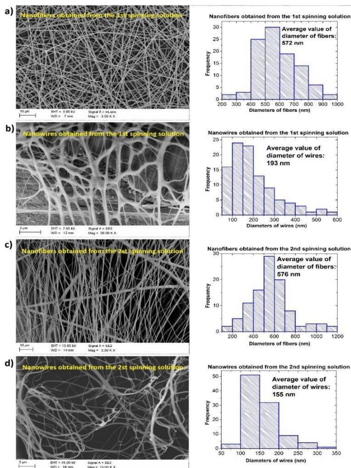
**Figure 1** Surface morphology images of the produced composite nanofibers PVP/SiO<sub>2</sub>, nanowires SiO<sub>2</sub> and histograms showing the distribution of the measured diameters of the tested nanomaterials: a), b) nanofibers and nanowires obtained the first spinning solution containing 1 ml of TEOS, c), d) nanofibers and nanowires obtained from the second spinning solution containing 4 ml.
