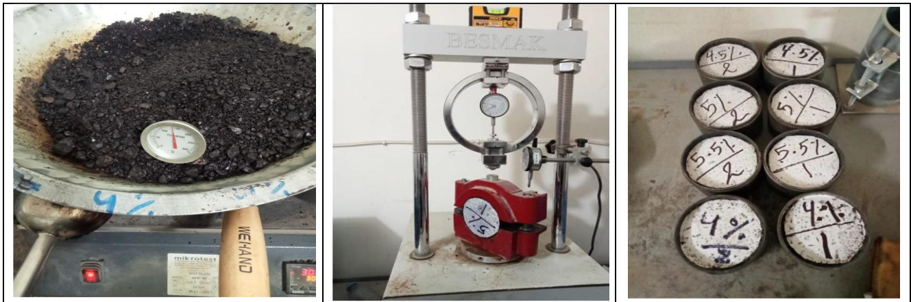
Figure 4 Samples of Asphalt Mixture by Marshall Test.
