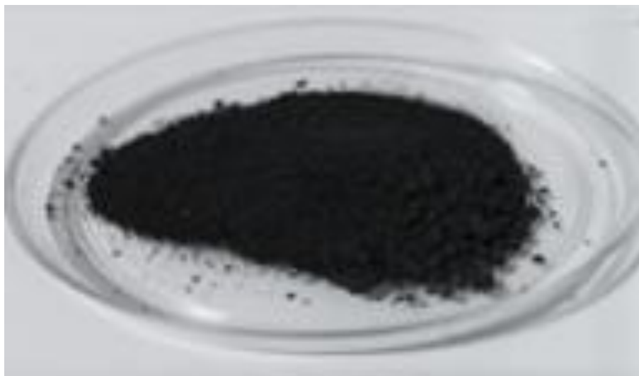
Figure 1 Powder of \text{NiMn}_2\text{O}_4 Calcined at 700 °C.
