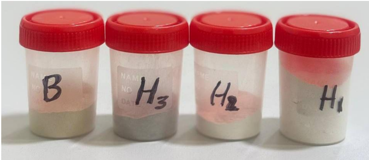
Figure 2 Digital photograph showing the color transition of bone powder from 600 °C to 1000 °C.
