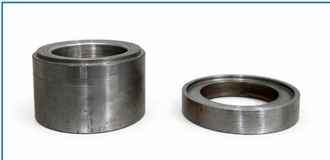
Figure 5 Photograph of the fabricated conical die and inclined blank holder with an inclination angle of 12^\circ used in the deep drawing experiments.
