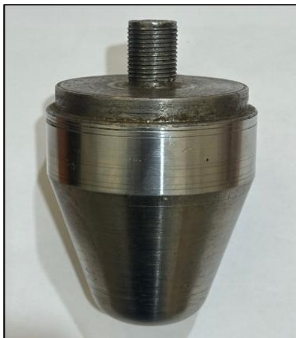
Figure 6 Photograph of the conical punch with a wall angle of 70^\circ employed for the fabrication of conical cups.
