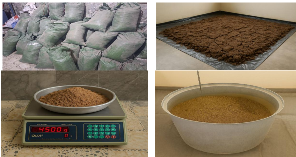
Figure 1 Sequential Protocol for Soil Sampling, Air-Drying, Mechanical Grinding, and Sample Homogenization.
