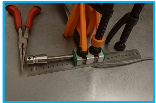
Figure 5 LVDT calibration process.
