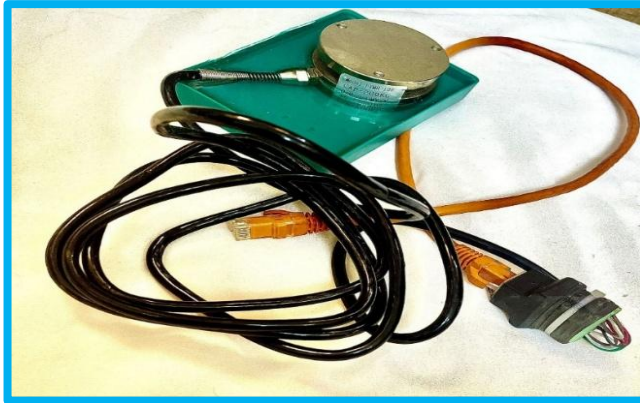
Figure 4 Soil pressure sensor under the pile tip.
