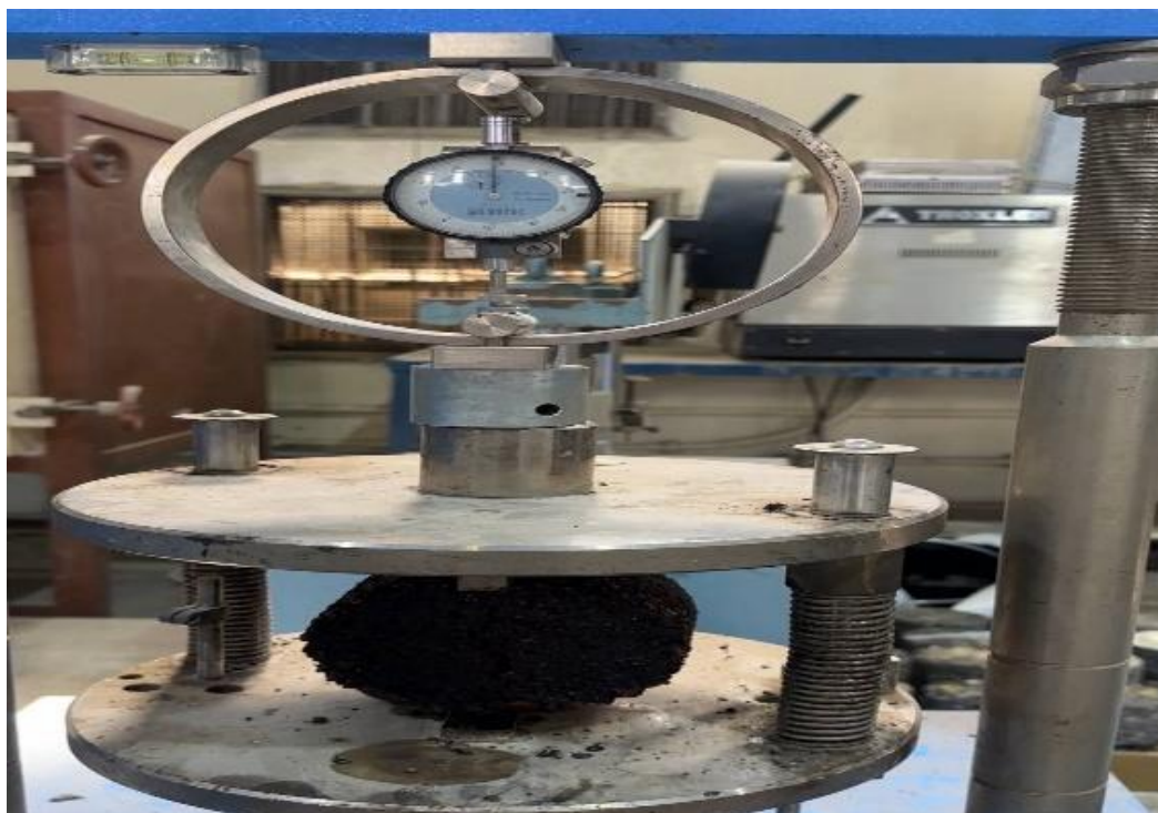
Figure 3 indirect tensile strength apparatus.
