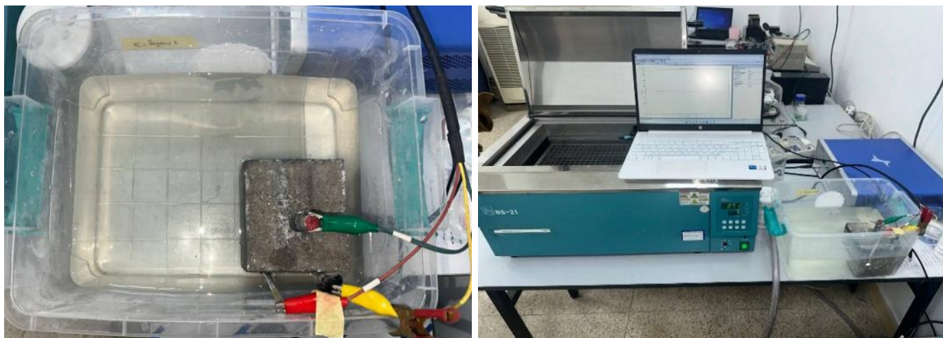
Figure 4 The electrochemical cell used for corrosion resistance measurement.
