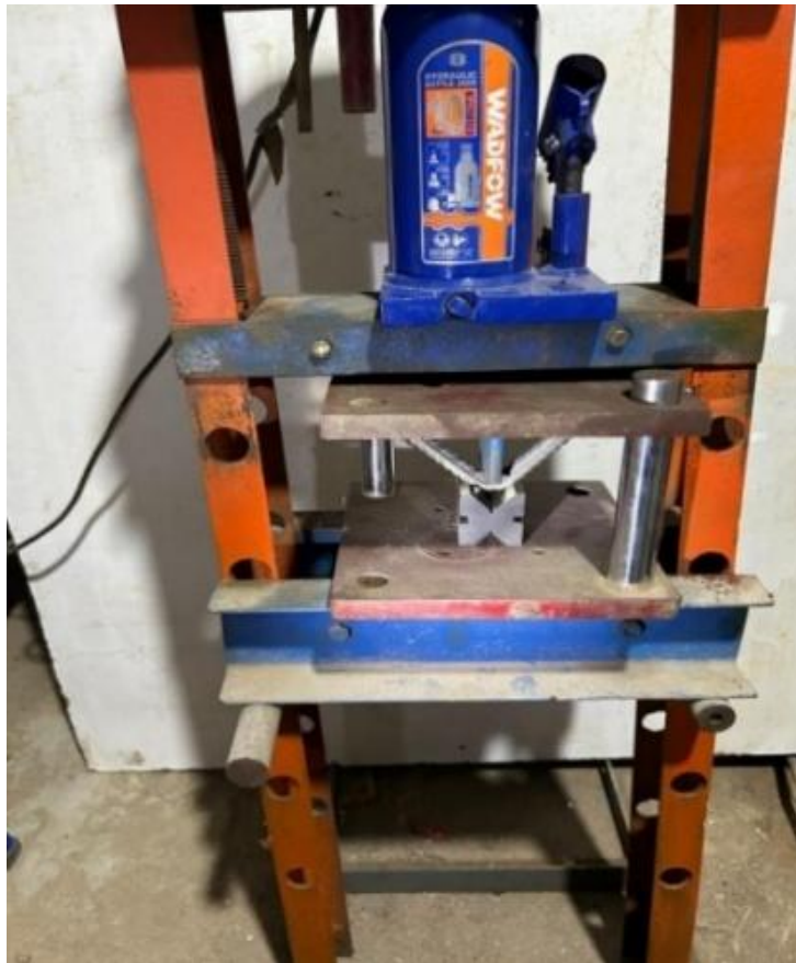
Figure 3 Coated sample during the bending process.
