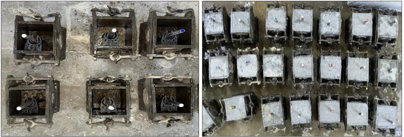
Figure 1 Concrete molds before and after casting.
