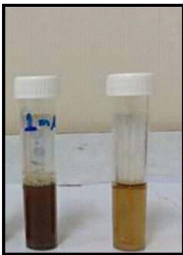
Figure 1 Silver nanoparticle (AgNP) solution (a) before and (b) after Ag NPs synthesis.
