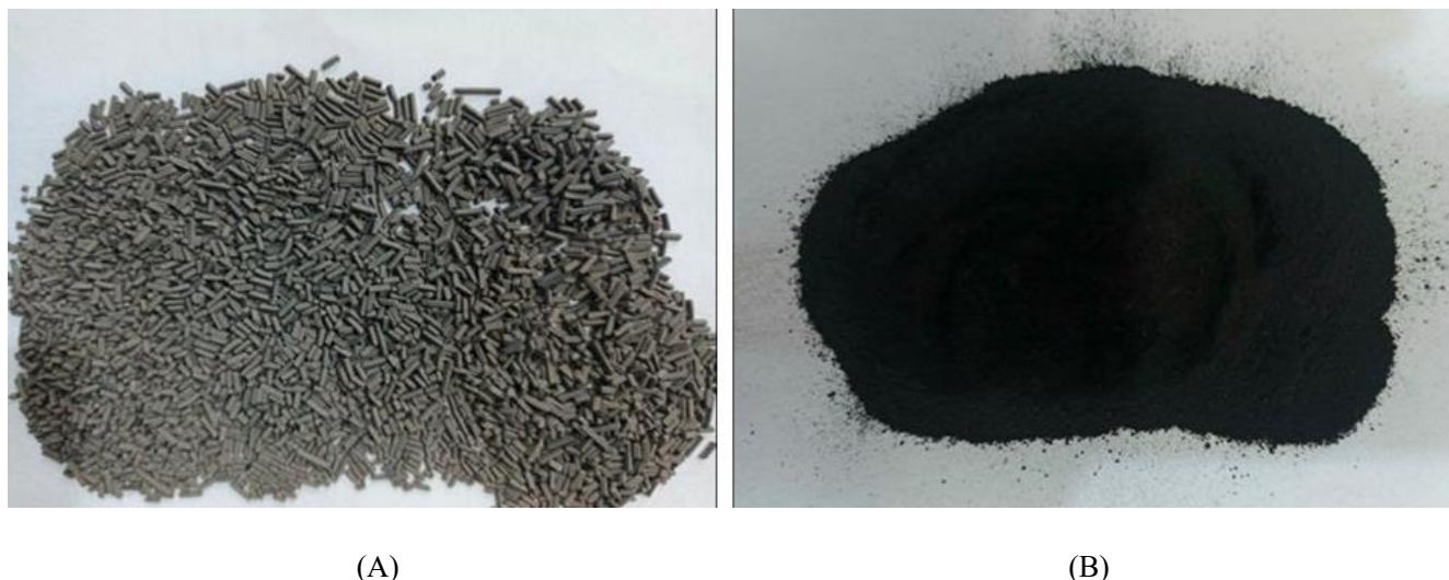
Figure 1 Spent CoMo/ \gamma -Al 2 O 3 , (A) Before and (B) After grinding.
