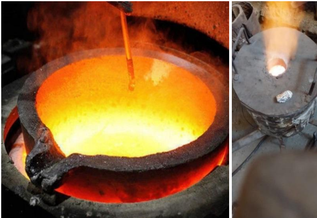
Figure 2 Melting process of Al6063 alloy.
