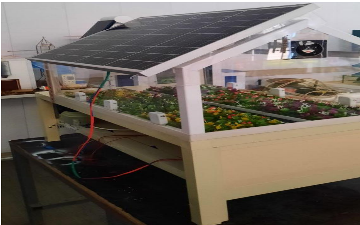
Figure 1 Greenhouse with Solar water heater system accompanies.
