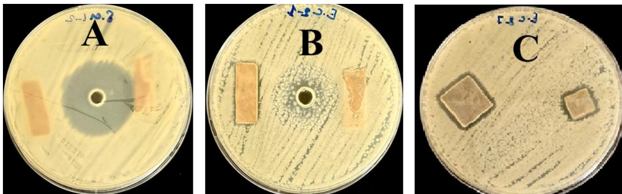
Figure 4 Zone of Inhibition (ZOI) results demonstrating the antibacterial efficacy against S. aureus for the coated samples, where the clear zones (A and B) indicate the potency of AgNPs in inhibiting microbial growth.
