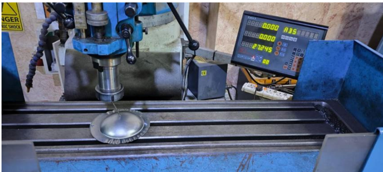
Figure 5 Measurement of dome height using NC milling machine (MF1 Farsmachine).
