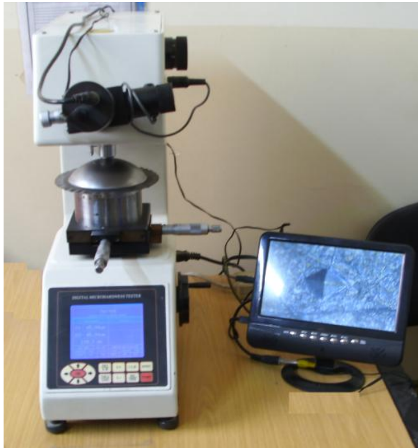
Figure 4 Digital micro-Vickers hardness testing machine used in this study.
