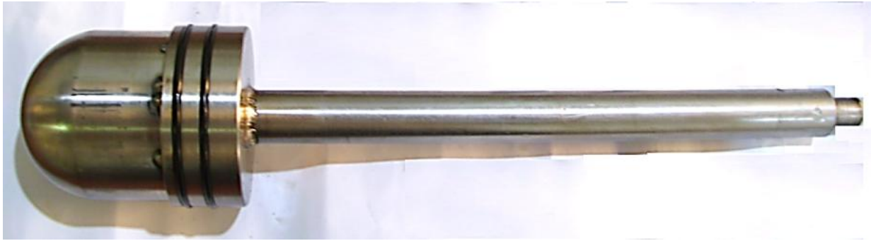
Figure 3 Hemispherical punch (Steel 45) welded to the piston for Nakazima formability test.
