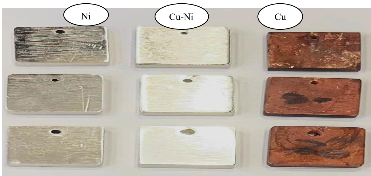
Figure 5 The samples after ELP, with different layers (Ni, Cu, Cu-Ni).
