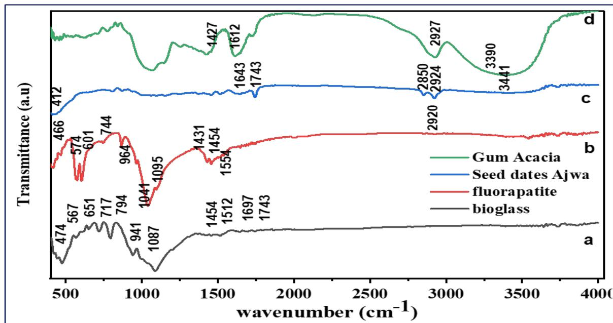
**Figure 3** FTIR spectra of resulted samples a) Bioactive glass, b) Fluorapatite, c) Ajwa Dates Seed and d) Gum Arabic.
