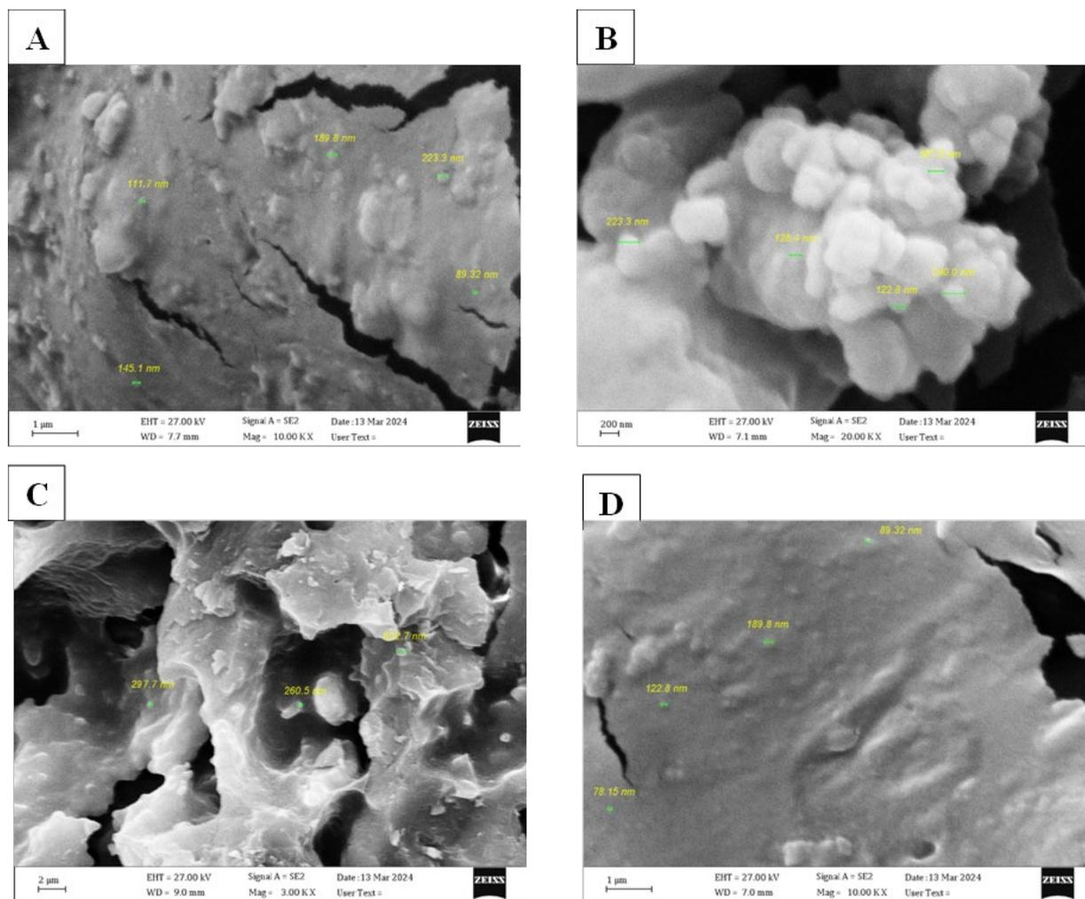
**Figure 4** (A-D) FE-SEM images of hybrid biocomposites Grafting Samples with different magnification A) Pure (BG-DS) NPs at 1μm. B) (5% FA-BG-DS) NPs at 200 nm, C) (15%FA-BG-DS) NPs at 2μm, and D) (25%FA-BG-DS) NPs at 1μm.
