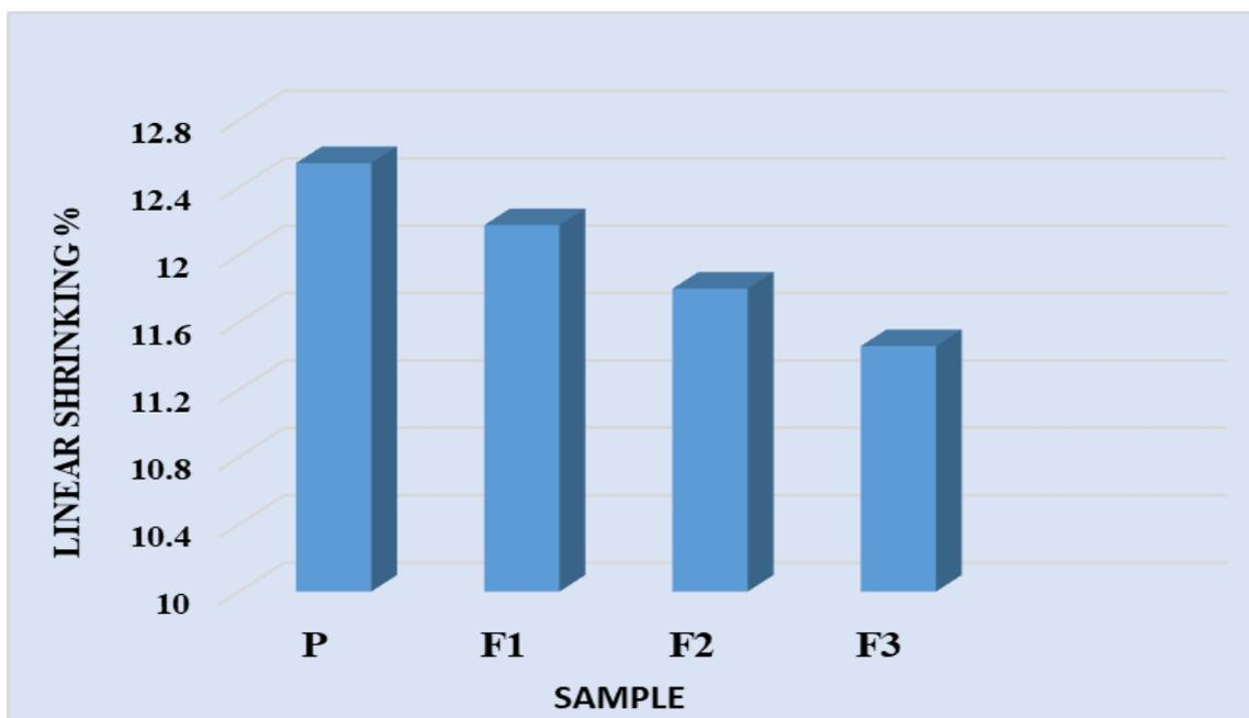
**Figure 6** Linear Shrinkage of All hybrid biocomposites Samples.
