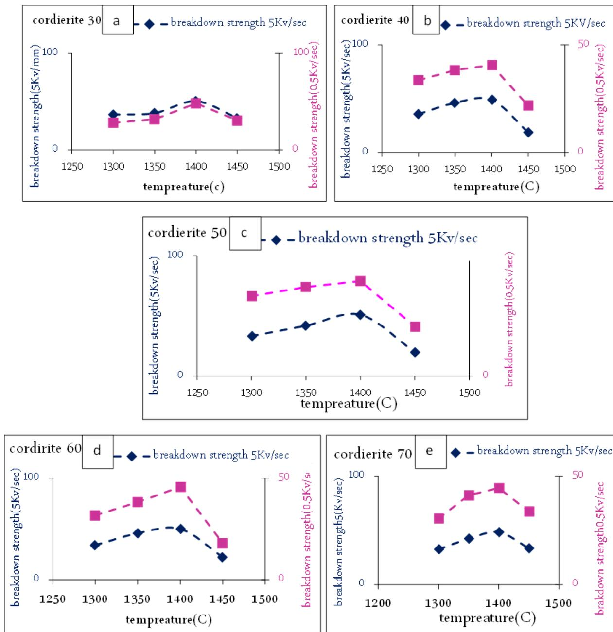
Figure 7 (a), (b), (c), (d) and (e) the relationship of the Breakdown strength with changing burning temperatures.
