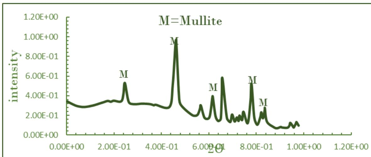
Figure 3 X- ray diffractograms mullite.
