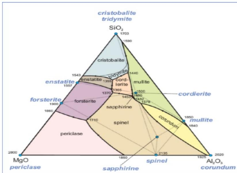
**Figure 2** Silica-alumina-magnesia system and the location of cordierite mineral.
