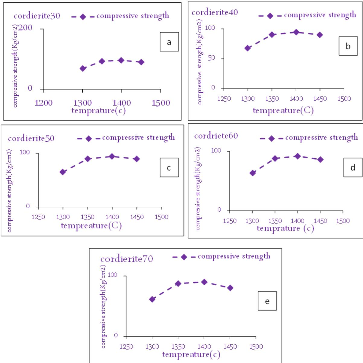
**Figure 6** (a), (b), (c), (d) and (e) the relationship of the compressive resistance with changing burning temperatures.
