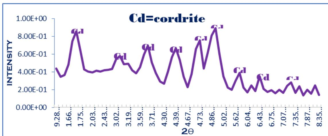
Figure 4 X- ray diffractograms cordierite.
