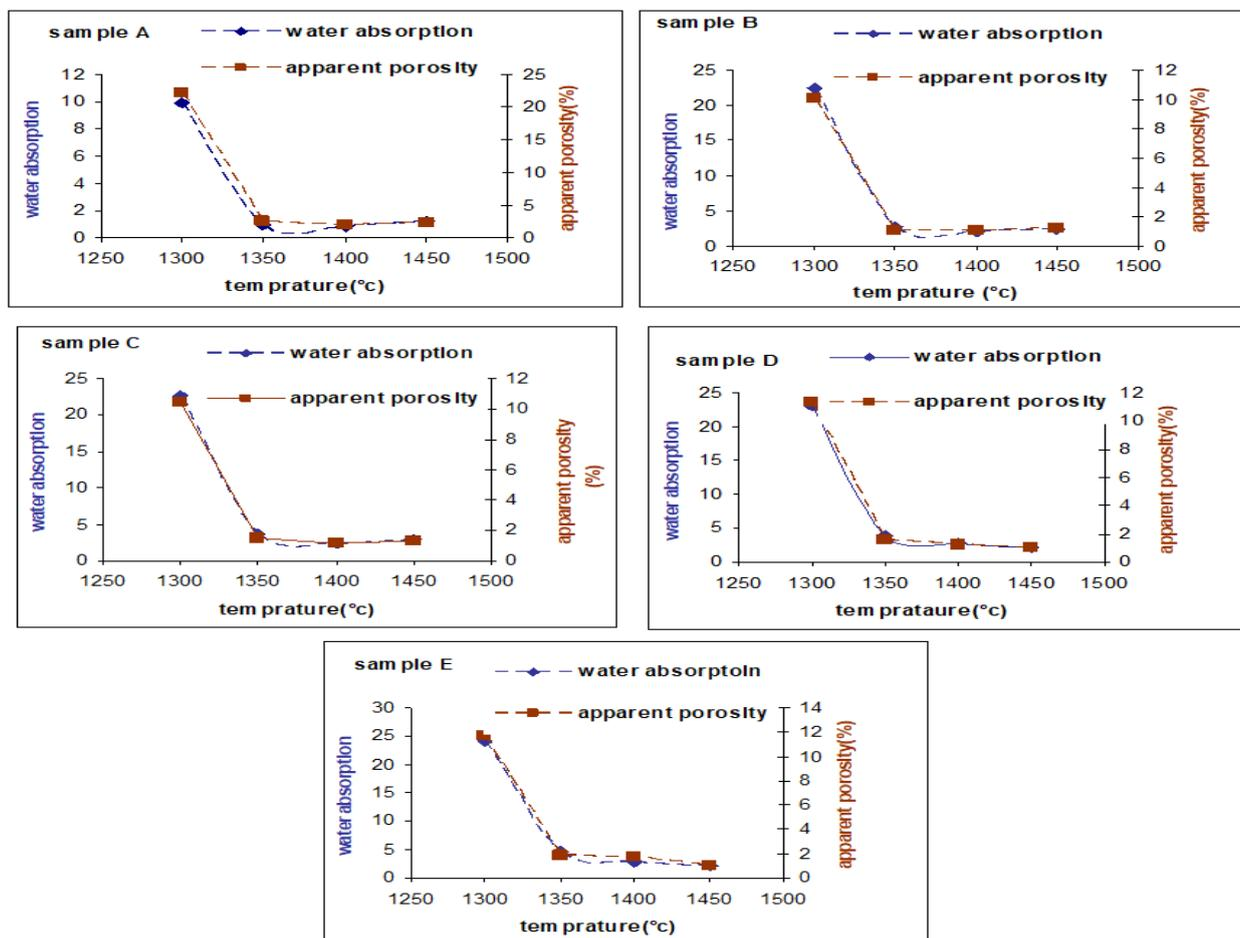
**Figure 5** (A), (B) , (C) , (D) and ( E) The relationship of the water absorption and apparent porosity with changing burning temperatures.
