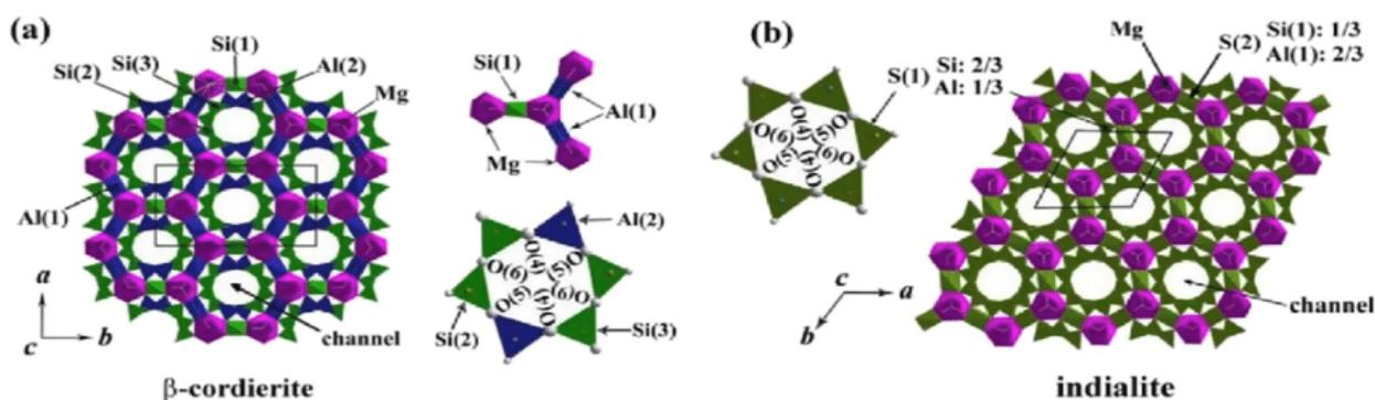
**Figure 1** Structure of cordierite when (A) low temperature, (B) heigh temperature.
