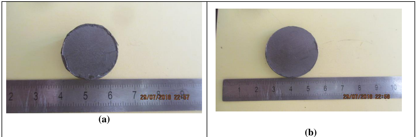
Figure 1 Sintered samples with die diameter of 20 mm: (a) Ceramic carbide A, (b) Composite Ceramic-Metal A or cermets.
