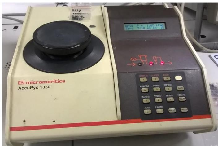
**Figure.6:** The measurement of the relative density.
