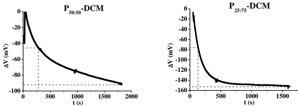
Figure. 6:  $\Delta V$  and  $t_{50}$  for copolysiloxane LB thin films,  $P_{50:50}$  and  $P_{25:75}$  with  $\text{CHCl}_3$ , IPA and DCM
