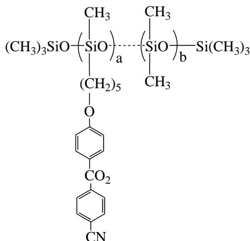
Figure. 1: General structure of copolysiloxanes, P<sub>50:50</sub> (a:b = 50:50) and P<sub>25:75</sub> (a:b = 25:75).
