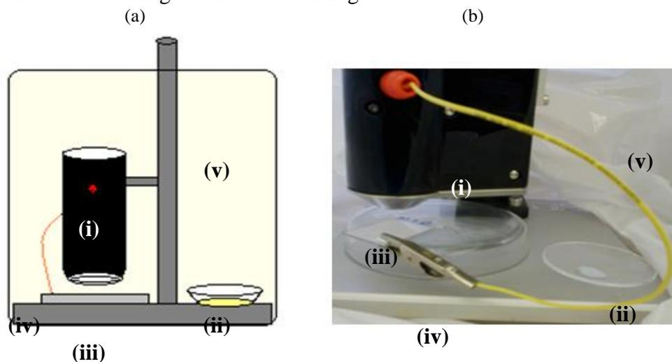
Figure. 4: Surface potential measurement setting in (a) diagram of the whole experimental setup and (b) actual experiment setup. Labels are (i) NIMA S-POT probe, (ii) solvents contained in a watch glass, (iii) LB thin film, (iv) Metal contact and (v) sealed bag.
