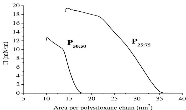
Figure. 5: Isotherm graphs of P<sub>50:50</sub> and P<sub>25:75</sub>.
